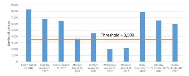
The daily automobile volume by access location is shown on Figure 6. On days without a cruise ship call, the parking lot at the West Gate is locked, and the small number of trips that entered or exited the terminal at the West Gate are likely related to security or maintenance personnel. Days with the largest number of vehicles accessing Terminal 91 correspond to days with cruise ship activity.
